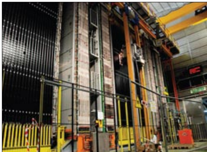
Figure 1. The OPERA detector system at LNGS in Italy. The black rack to the left is a stack of 150,000 8.3 Kg (~18 pound) bricks of photographic film interleaved with lead sheets and plastic scintillators to count and time-stamp the arriving neutrinos. 5
